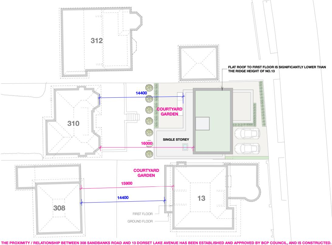
AS SHOWN IN THE DRAWING ABOVE, THE DISTANCE BETWEEN THE RESPECTIVE FIRST FLOORS OF 308 SANDBANKS ROAD AND 13 DORSET LAKE AVENUE IS 15.9m. THE DISTANCE BETWEEN THE FIRST FLOORS OF 310 SANDBANKS ROAD AND THE PROPOSAL IS 16m. THE PROPOSED GROUND FLOOR EXTENDS BACK FURTHER THAN NO. 13 GROUND FLOOR, ALTHOUGH THIS IS SINGLE STOREY ONLY AND WILL NOT HAVE ANY MATERIAL OVERBEARING IMACT ON ANY SURROUNDING PROPERTY.
